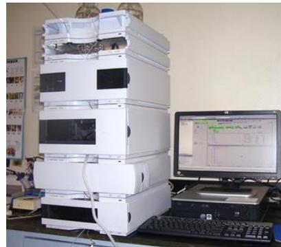
Appareil de CLHP-UV/HPLC-UV
