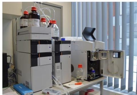
Appareil de CLHP-SM/HPLC-MS
